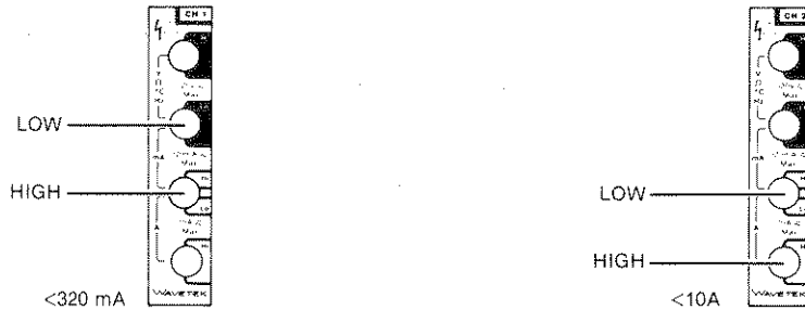
Figure 6-4. Current Input Connections
